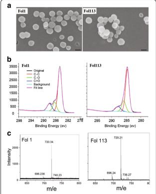
**Fig. 1** The physiochemical characterizations of fullerenols. **a** SEM images of NP aggregates (bar = 100 nm), **b** XPS data, **c** MALDI-TOF-MS data without a matrix
